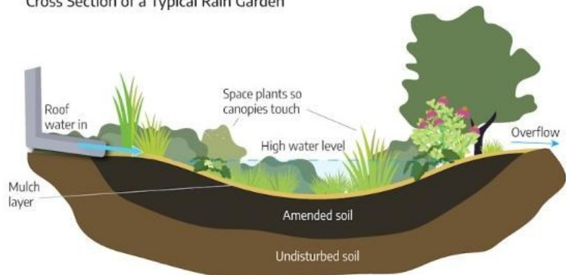
Cross Section of a Typical Rain Garden
